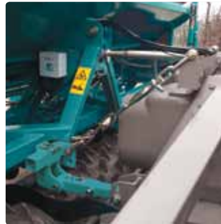
Triangle linkage on tools from other brands
