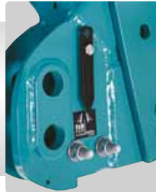
Level and angle indicator for late spreading
