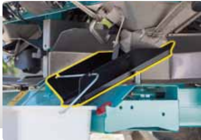
Emptying chute for calibration test
