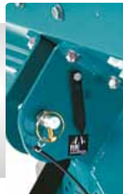
Level and angle indicator for late spreading
