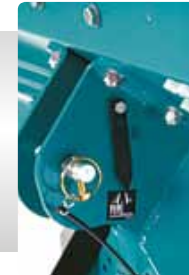
Level and angle indicator for late spreading
