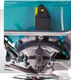
TRIBORD 2D: border device controlled from the cab
